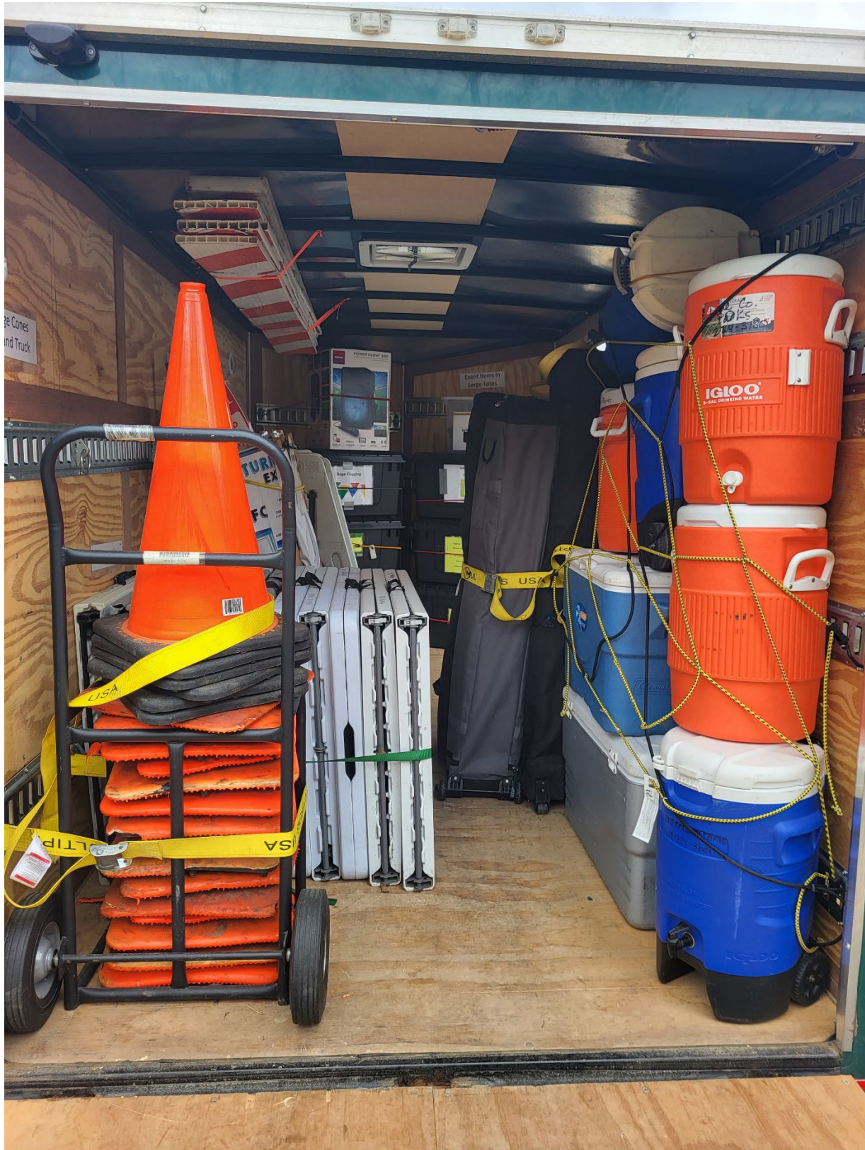
Back of trailer: Cones stacked neatly on dolly and secured to wall with yellow ratchet strap. Coolers stacked neatly and secured with “octopus-style” bungee cord. Tables secured with small ratchet strap.
