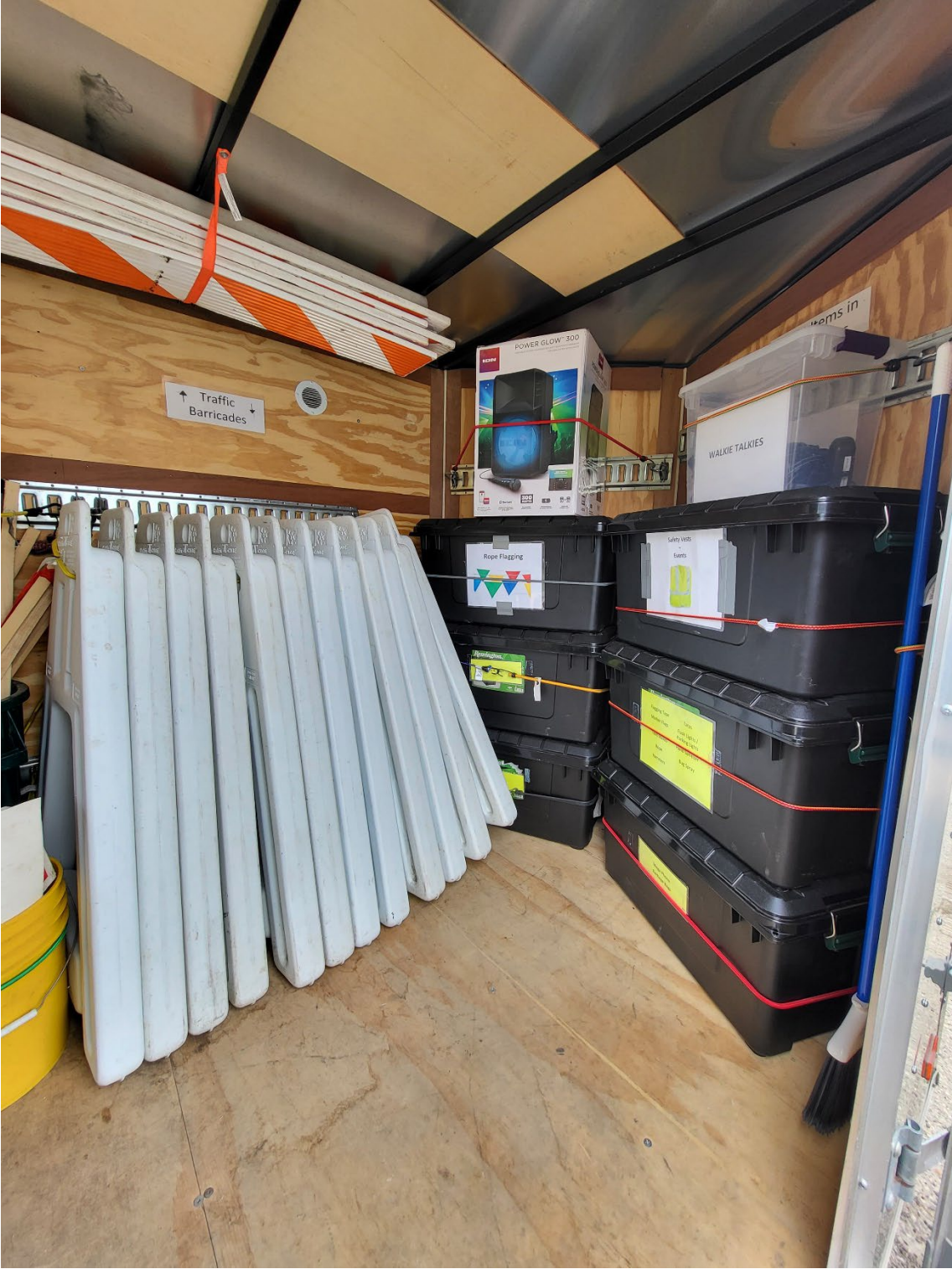
Front of Trailer: Smaller boxes stacked on top of large, everything secured with bungee cords. Parking barricades: “feet” secured by bungee cords; top “bars” secured by two small orange ratchet straps attached to ceiling (make sure they are re-tightened when the bars are put back).
